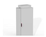
This roof air-water heat exchanger, PWD, with a IP 55 protection degree, is ideal for dusty environments with high temperatures. Air cleanliness and the temperature around the enclosure will not affect the heat exchanger's performance. Floor standing enclosures may be cooled independently, if needed, which reduces energy consumption. The heat exchanger is placed on top of the enclosure, which means cooling can be provided also when there is not enough space on the door or side panels.
